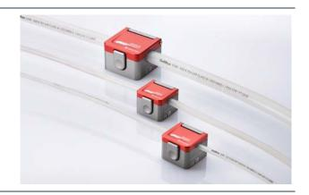
SONOFLOW CO.55 V3.0 clamp-on flow meters measure the flow rate of liquids in flexible tubes of different diameters. With high accuracy, reproducibility and repeatability – even in the lowest flow range – the sensors are suited for a variety of applications. Various accessories allow for easy integration into bench top setups and industrial process environments.
