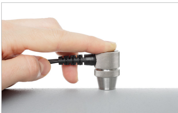
Wall thickness gauge NT in use
