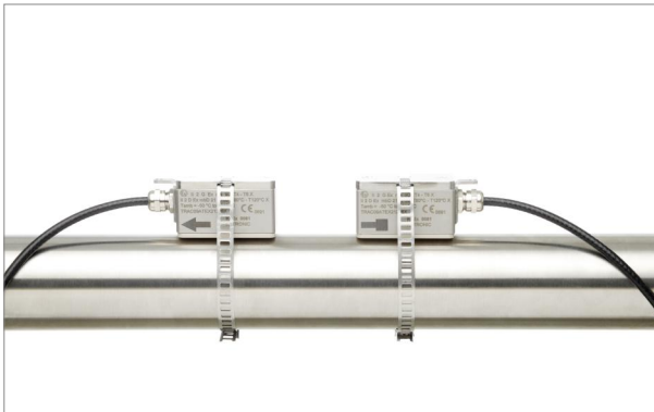
K1Ex transducers mounted using straps and clamps
