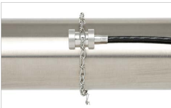
PT100 transducer fixed to pipe
