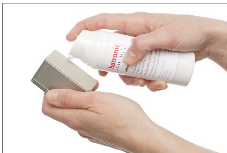
Picture 9: Application of acoustic coupling gel
