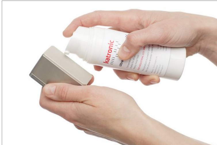
Picture 7: Application of acoustic coupling gel
