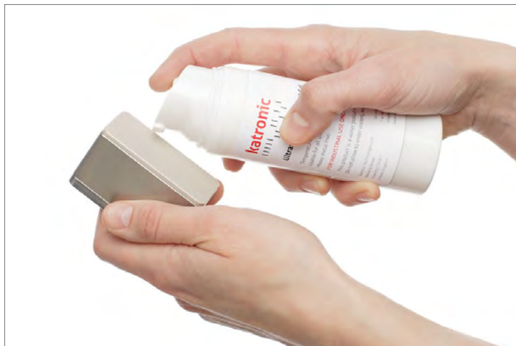
Picture 8: Application of acoustic coupling gel
