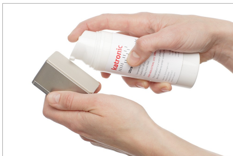
Picture 8: Application of acoustic coupling gel
